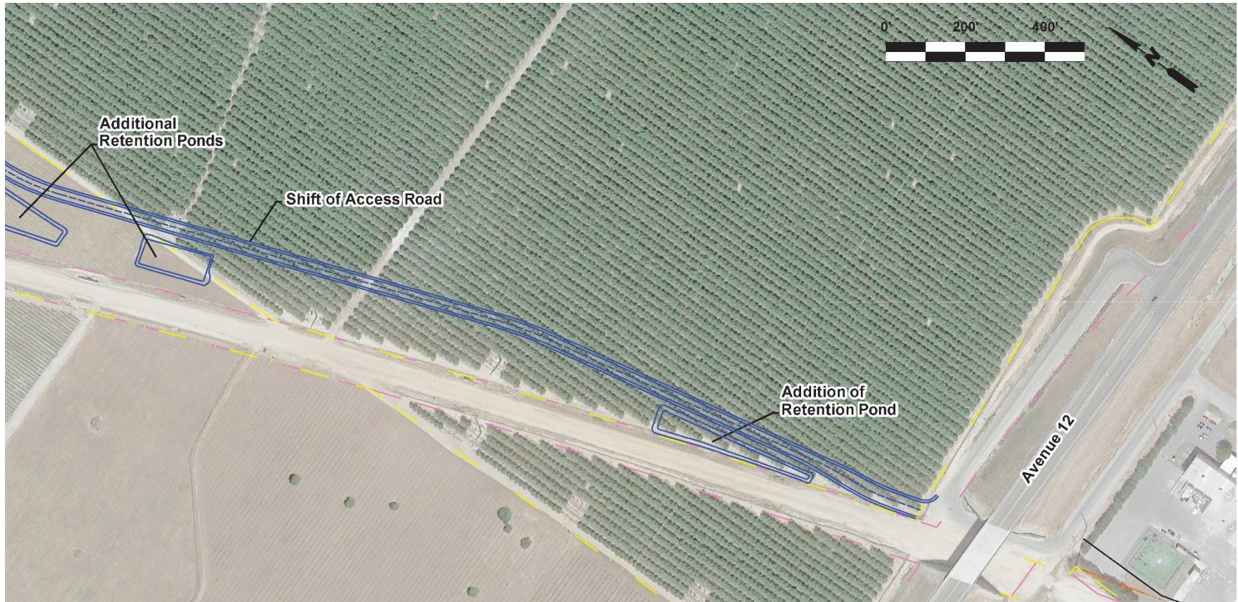
Figure 2-5. Updated Phase 1 Project Elements – Access Road
